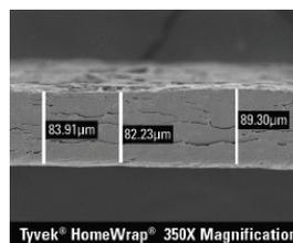
not a hybrid combination of multiple materials. It is 100% high-density flashspun polyethylene so weather resistance and durability runs through the entire thickness of the product.
